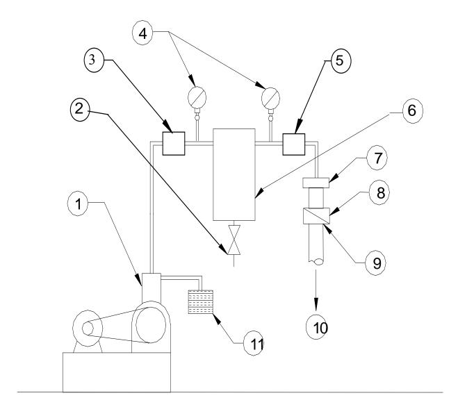
Figure 44. Individual Compression-Type Air Supply
