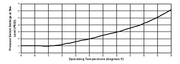
Figure 57. Pressure Switch Setting
