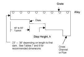
Figure 2. Stepped Gravity Flow Gutter
