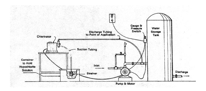
Figure 30. Positive Displacement Chlorinator
