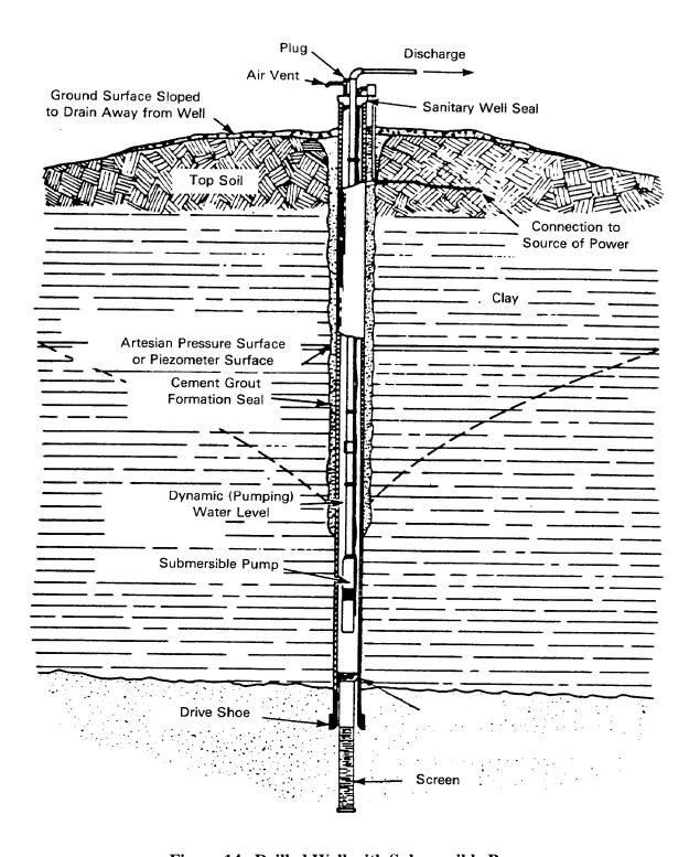
Figure 14. Drilled Well with Submersible Pump
