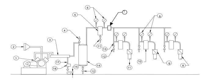
Figure 45. Central Compression-Type Air Supply
