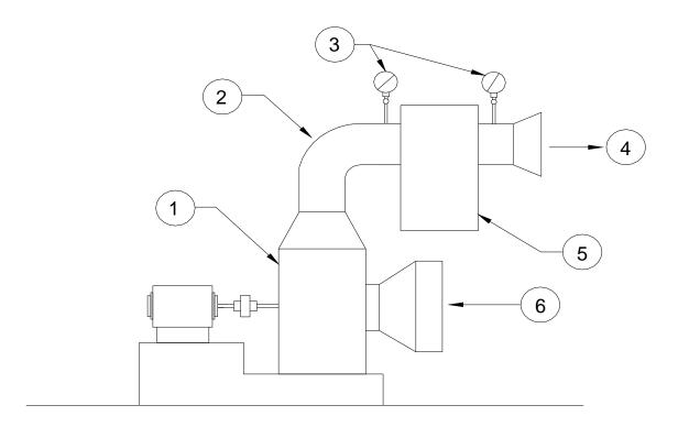
Figure 46. Individual Blower-Type Air Supply
