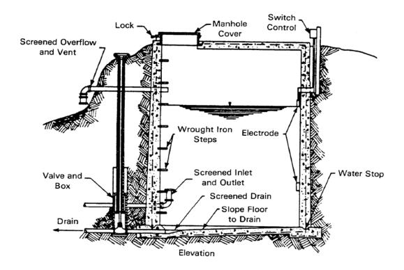
Figure 21. Typical Concrete Reservoir
