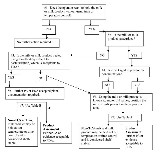
Figure 59. Decision Tree for Using pH, a<sub>w</sub>, or the Interaction of pH and a<sub>w</sub> to Determine if a Milk or Milk Product Requires Time/Temperature for Safety
